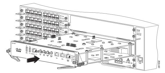
Step 4 Carefully slide the module into the slot until the EMI gasket on the module makes contact with the module in the adjacent slot and both the ejector levers have closed to approximately 45 degrees with respect to the module faceplate.
